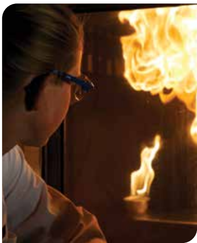
Once ignited, organic peroxides burn more violently than common solvent like, for example, acetone.
