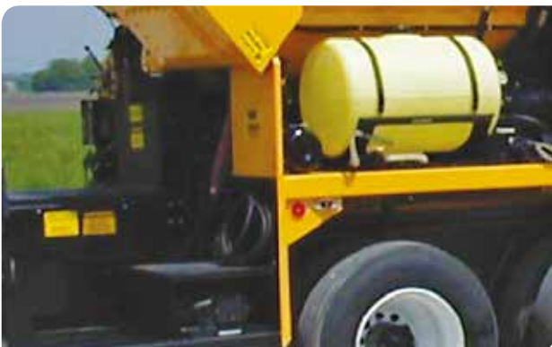
Additive tank on the paver Additive is used to extend the mix time in hot weather
