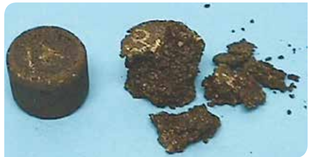
In the Schultze Breuer Ruck test small "pills" prepared from the slurry ingredients in fixed proportions are subjected to water soak and abrasion, eventually in boiling water, and the damage assessed on a points scale
