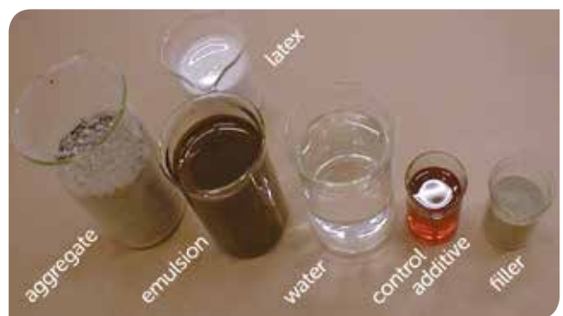
Slurry surfacing mix design components
