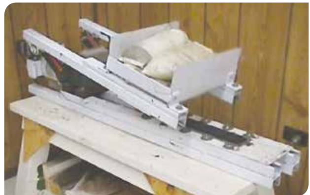
In the Schultze Breuer Ruck test small "pills" prepared from the slurry ingredients in fixed proportions are subjected to water soak and abrasion, eventually in boiling water, and the damage assessed on a points scale
