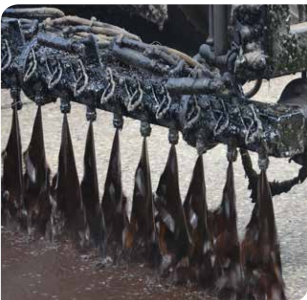
As observed, all spray nozzles were properly aligned and not clogged.
