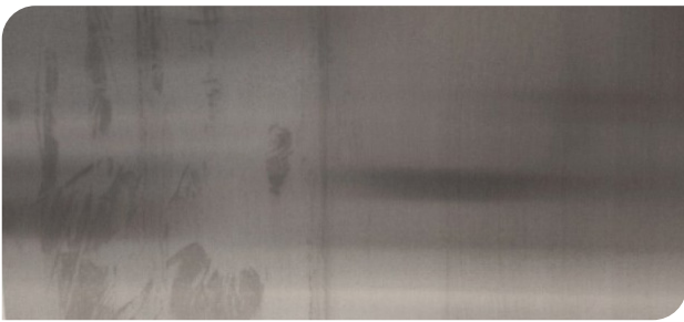
Stainless steel fingerprint test: untreated surface (left) vs Berol® LS surfactant treated surface (right) after wiping with a damp cloth.
