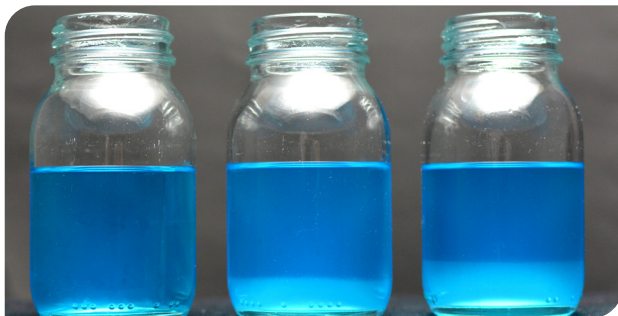
Finnfix® LD CMC no separation Best commercial CMC separation Regular purified CMC separation
