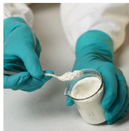
Expancel® DU Dry, unexpanded microspheres
