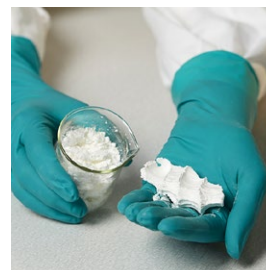
Expancel® WE Wet, expanded microspheres
