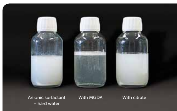
Figure 12: Ca soap scum formation of a liquid anionic soap in the presence of Ca 2+ ions and with MGDA or citrate addition.
