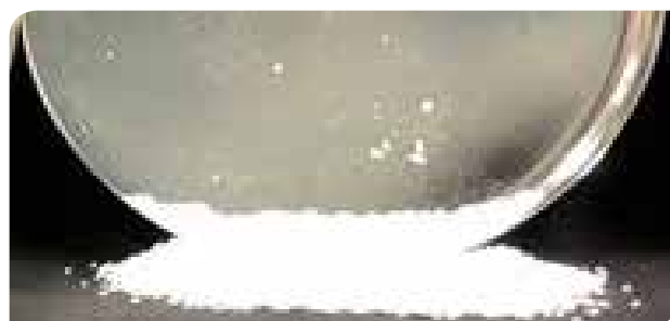
Figure 10: Petri-dish in vertical position with non-sticking Dissolvine ® M-S after storage at 65% Relative Humidity at 40°C
