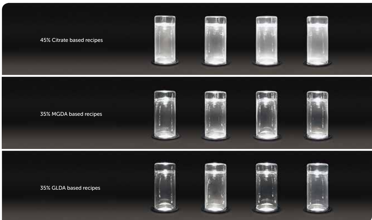
Figure 13: Anti-spotting and filming performance of several formulas based on citrate, MGDA and GLDA after 10 washing cycles.
