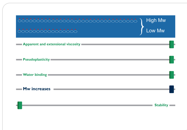
Figure 2. Descriptors function as equalizer and show the influence of the molecular weight on the CMC performance.
