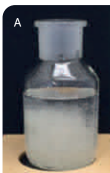
Figure 19: When a CMC particle enters water (A) it will go through a process of hydration by adsorption of water. Particles swell (B) and increase in volume, as shown on the figures above. It is possible to reach even the higher viscosity levels compared to that of the final solution due to higher amount of water bound in this state. It is important to wait until the viscosity is stabilized to reach stable dissolution (C). Dispersion means a uniform distribution of the CMC particles in water. Solution means that the CMC is completely dissolved in water.
