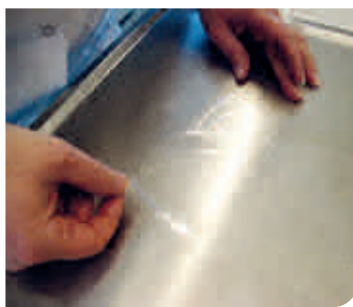
Figure 17: CMC forms an oil and grease resistant film on a substrate, which can be used in food packaging. Bio-based and biodegradable solutions are developed to meet the increasing demand for sustainable packaging.
