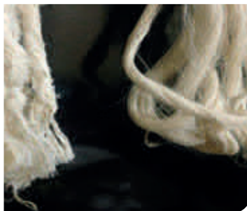
Figure 18: Sizing of warp yarns with FINNFIX CMC increases the yarn strength providing the opportunity to increase weaving efficiency. CMC creates a strong, abrasion-resistance film that exhibits good adhesion especially to the cotton fiber surface and also reduces dusting.
