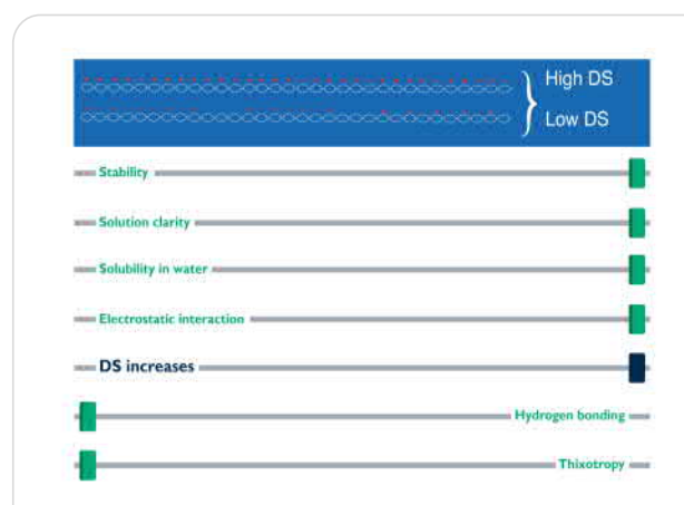
Figure 4: Descriptors function as equalizer and show the influence of the DS on the CMC performance.
