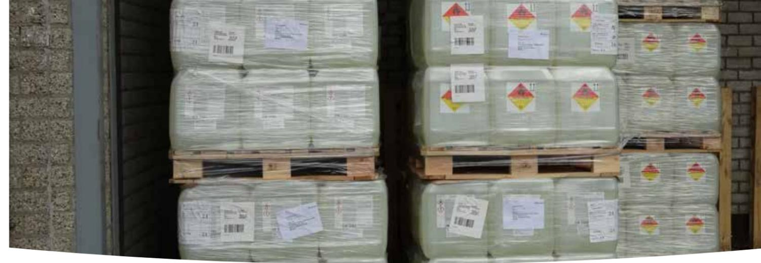
Space between pallets to allow maximum air circulation
