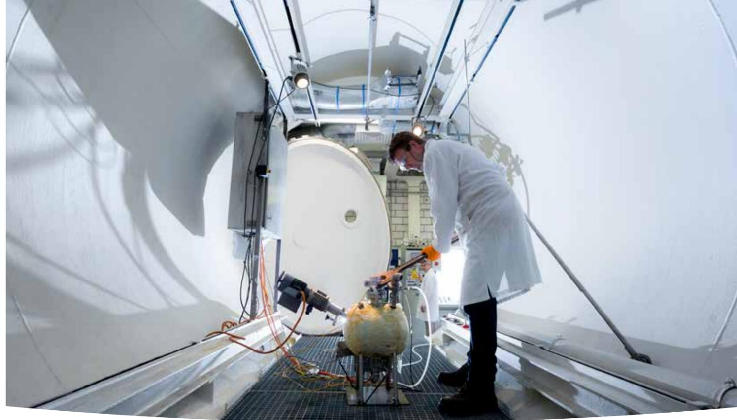
55 m<sup>3</sup> total containment tank for large-scale safety testing in Deventer, the Netherlands
