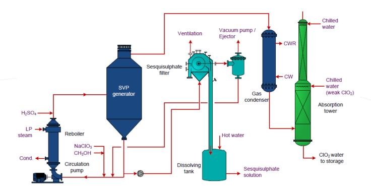
The key feature of the SVP-LITE<sup>®</sup> process is the circulation of the main reactor vessel, which is kept under vacuum:
