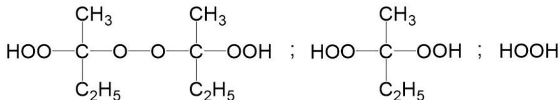
Cadox® D-50 VRN is a multipurpose catalyst used for curing gel coats and promoted unsaturated polyester resins at room temperature.
