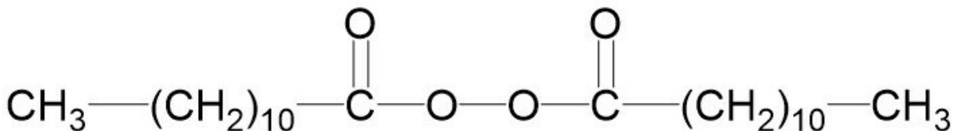
Laurox S is an initiator for (co)polymerization of styrene, ethylene, vinyl chloride, vinylidene chloride and (meth)acrylates. Possible to store at ambient temperatures.
