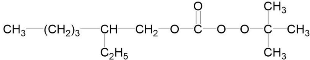
Trigonox® 117 can be used to crosslink elastomers at intermediate temperatures, a typical crosslink temperature is 150°C. Trigonox® 117 is recommended for highly demanding applications e.g. as crosslinker for the ethylene vinylacetate copolymer (EVA) film in photovoltaic devices.
