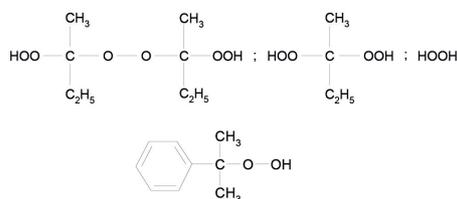
Trigonox 289-IN VRN is a special peroxide blend with a VRN system, suitable for curing unsaturated polyester and vinyl ester resins at ambient conditions in conjunction with a metal accelerator.
