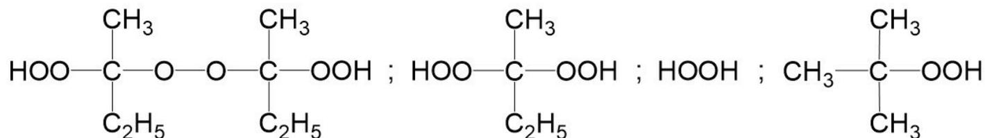
Trigonox® 82 is a peroxide mixture, specially developed for the production and cure of thick laminates (>15 mm) in one operation and for those applications where a high peak exotherm should be avoided. Application: pipes, tanks, windmill rotors.
