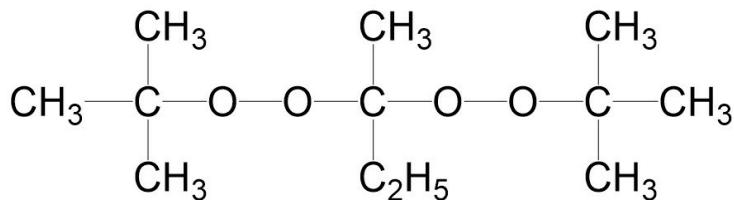
Initiator (50% active ingredient in mineral oil) for (co)polymerization of (meth)acrylates.
