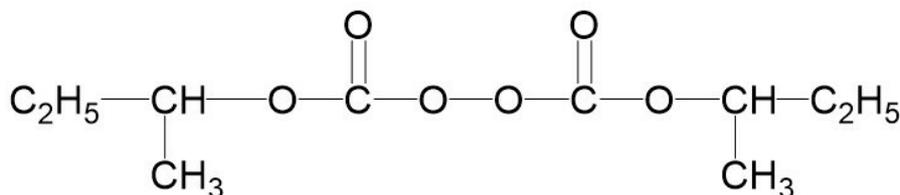
Trigonox® SBP is an initiator for (co)polymerization of ethylene, vinyl chloride and vinylidene chloride.
