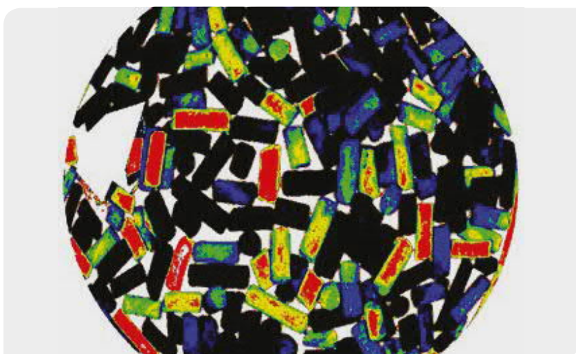
Figure 1. Normalized SEM-BSE image of a hydrogenation catalyst, showing the variation in metal loading between and on extrudates (black = low loading; red = high loading)
