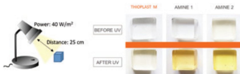
Figure 5. Schematic representation of the experimental setup (left). Test specimen before and after 14 days of exposure to UV light.
