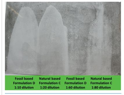
Fig. 2 Black box cleaning test of a coated metal tile soiled with diesel train engine soil and aged for 12 hours at room temperature.
