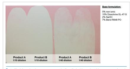
**Fig.1** Black box cleaning test on a ceramic tile soiled with used cooking grease and aged for 5 hours at 60°C.
