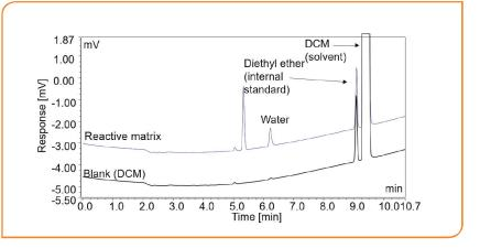
Figure 2: GC chromatogram of a reactive sample containing 0.5 mass % of water
