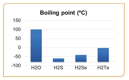
Figure 1: Influence of hydrogen bonding on boiling point
