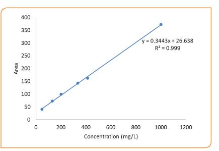
Figure 3: Calibration line of water; with Diethyl Ether as internal standard
