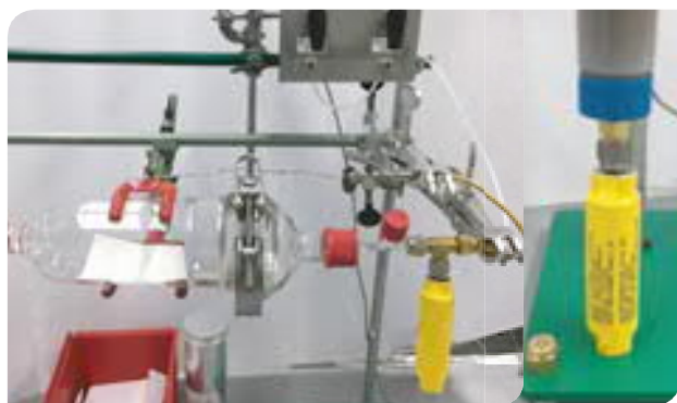
Figure 1: Adsorption test set-up consisting of glass exposure chamber and permeation device (yellow tube)
